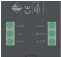
As the LEDs have been designed for quick immediate diagnosis, the status of each input and output is highlighted by one specific LED. This makes it possible to quickly identify the interruption points in the safe chain, which device is released, which door is opened and any errors inside the device. All that in a straightforward way without needing to decode complex blinking sequences.
