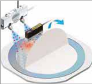
Measuring surface potential when removing BG sheets
