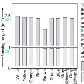
These bars indicate the sensing range with the respective colors when the distance adjuster is set to a sensing range of 2.5 m 8.202 ft / 1 m 3.281 ft long, respectively, with e non-glossy paper. The sensing range also varies depending on material.
