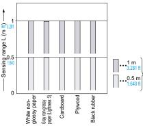
These bars indicate the sensing range with the respective objects when the distance adjuster is set to a sensing range of 1 m 3.281 ft / 0.5 m 1.640 f long, respectively, with white non-glossy
