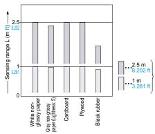
These bars indicate the sensing range with the respective objects when the distance adjuster is set to a sensing range of 2.5 m 8.202 ft / 1 m 3.281 ft long, respectively, with white non-glossy paper.
