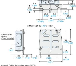
Material: Cold rolled carbon steel (SPCC)
