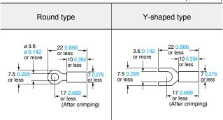
Note: Use crimp terminals with insulating sleeves.
