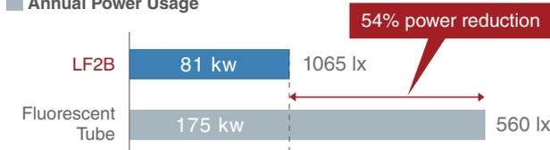
Note: Comparison of LF2B-D3 (580mm) and fluorescent tube (580mm).
