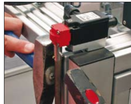
Switch locking (pin provided).
