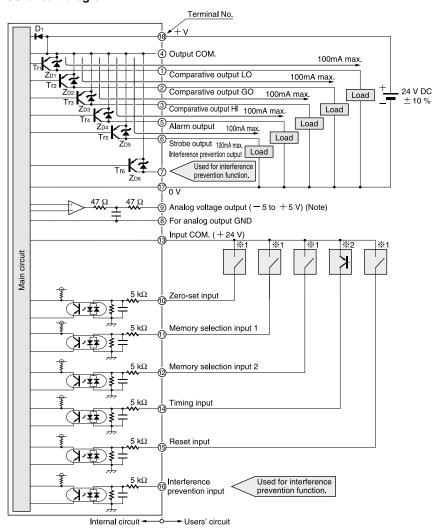
Note: Devices connected to the analog voltage output must have an input impedance set at 1  $\mbox{M}\Omega$  or more.
