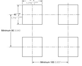
Note: The panel thickness should be 1 to 2.5 mm 0.039 to 0.098 in.
