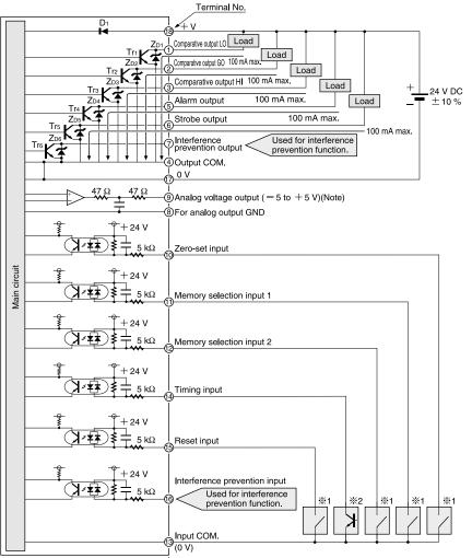
Note: Devices connected to the analog voltage output must have an input impedance set at 1  $\mbox{M}\Omega$  or more.
