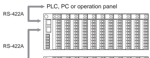
Up to 16 units (Max. 320 loops) are available when connected to a RKC touch screen operation panel, PLC or a host computer.
