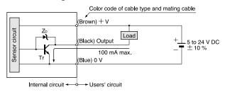
Note: Make sure to connect terminals correctly as the sensor does not incorporate a reverse polarity protection
