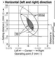
The sensors can be mounted side by side. However, if the sensor is slanted, there may be interference. Verify first whether there is any interference prior to use
