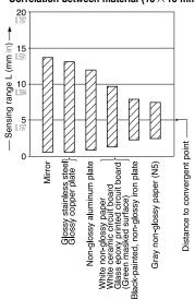
The bars in the graph indicate the sensing range for the respective material. However, there is a slight variation in the sensing range depending on the product. Further, if there is a reflective object (conveyer, etc.) in the background of the sensing object, since it affects the sensing, separate it by more than twice the sensing range shown in the left graph.
