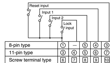
Note: The LC4H-W does not have the lock input ④ ⑦.
