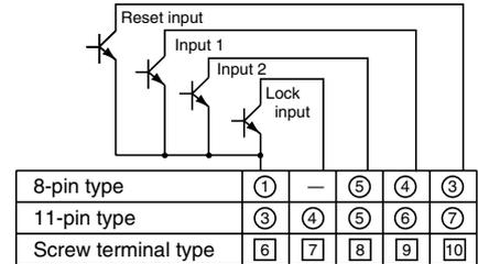
Note: The LC4H-W does not have the lock input ④ ⑦.
