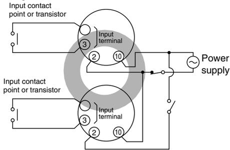
one input signal can be fed to two or more counters at once, as shown in Fig. C.
