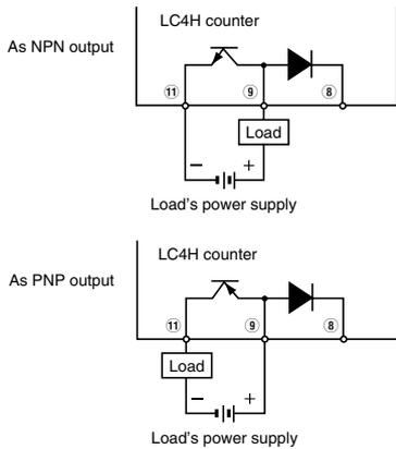
Note: With the LC4H 8-pin type and the LC4H-W, there is no diode between points ⑧ and ⑨.
