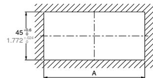
Note 1: The installation panel thickness should be between 1 and 5 mm .039 and .197 inch.
