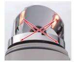
The uniquely designed reflectors not only reflect upward and to the side, but also downward; this cannot be achieved by incandescent bulb type revolving warning lights. The PATLITE LED revolving warning light is suitable for applications where high visibility from a low angle is required.
