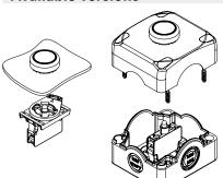
The LED holders of the control and signalling devices have two types of fixing: panel and base fixing.
